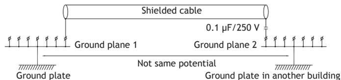
With longer distances, there is a risk that the ground potential may be different. In that case, the shield should only be connected at one end. A good alternative is to connect the other end of the shield to the ground via a  $0.1 \mu\text{F}/250 \text{ V}$  film capacitor. Both ends are then connected to the ground in terms of HF, but only connected to the ground at one end in terms of LF, thus avoiding the 50/60 Hz grounding loops.
