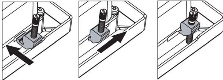
*Tighten the screws to 0.75 Nm*
