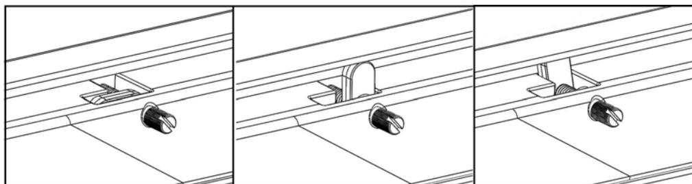
*Tighten the screws to 0.7 Nm*
