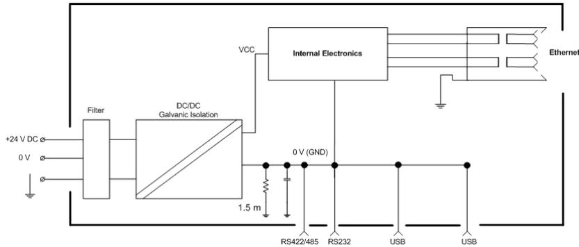
The operator panel has galvanic isolation against the 24 V DC power supply but no galvanic isolation between the communication ports for RS-232, RS-422/RS-485 and USB. Only the Ethernet connection has galvanic isolation.
