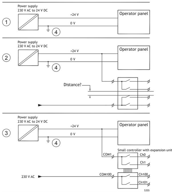
If a power supply that meets safety standards is used and only powers the operator panel, there is no problem. See 1 in drawing above.
