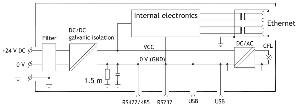
The operator panel has galvanic isolation against the 24 V DC power supply but no galvanic isolation between the communication ports for RS-232, RS-422/RS-485 and USB. Only the Ethernet connection has galvanic isolation.
