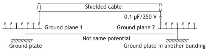
With longer distances, there is a risk that the ground potential may be different. In that case, the shield should only be connected at one end. A good alternative is to connect the other end of the shield to the ground via a 0.1 µF/250 V film capacitor. Both ends are then connected to the ground in terms of HF, but only connected to the ground at one end in terms of LF, thus avoiding the 50/60 Hz grounding loops.
