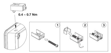
4. Connect the cables in the specified order, according to the drawing and steps below
