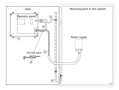
The mounting clamps of the operator panel do not provide a secure grounding connection between the panel and the device cabinet, see 1 in drawing above.
