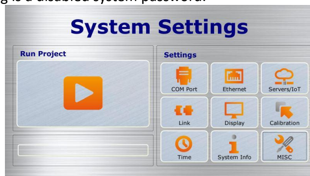
Figure 461 System Setting home page for HMI
