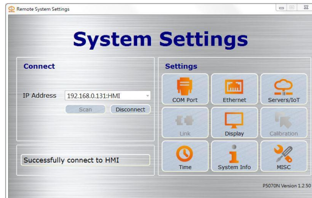
Figure 442 【 Remote System Setting 】 successfully connect to HMI
