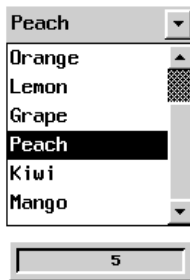
The Drop Down List object and the display of the register value of the item
