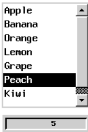
The List object and the display of the controller register value of the item
