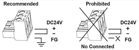
HMI unit and other equipment should have the same electrical grounding (reference voltage level), otherwise communication errors may occur.
