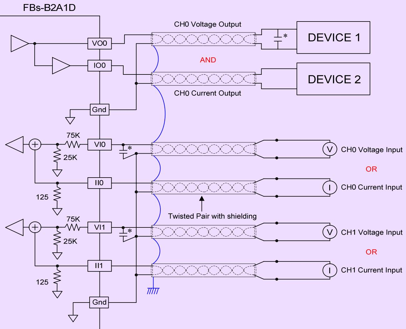
\* 0.1~0.47 uF capacitor ( to filter noise ) .....Advice to Install, but not necessary!!
